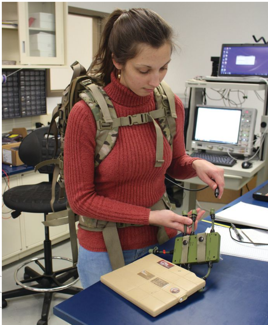
The Integrated Soldier Power and Data System, demonstrated here by an Army engineer, harvests energy to charge a battery that powers soldiers' wearable electronic equipment.
