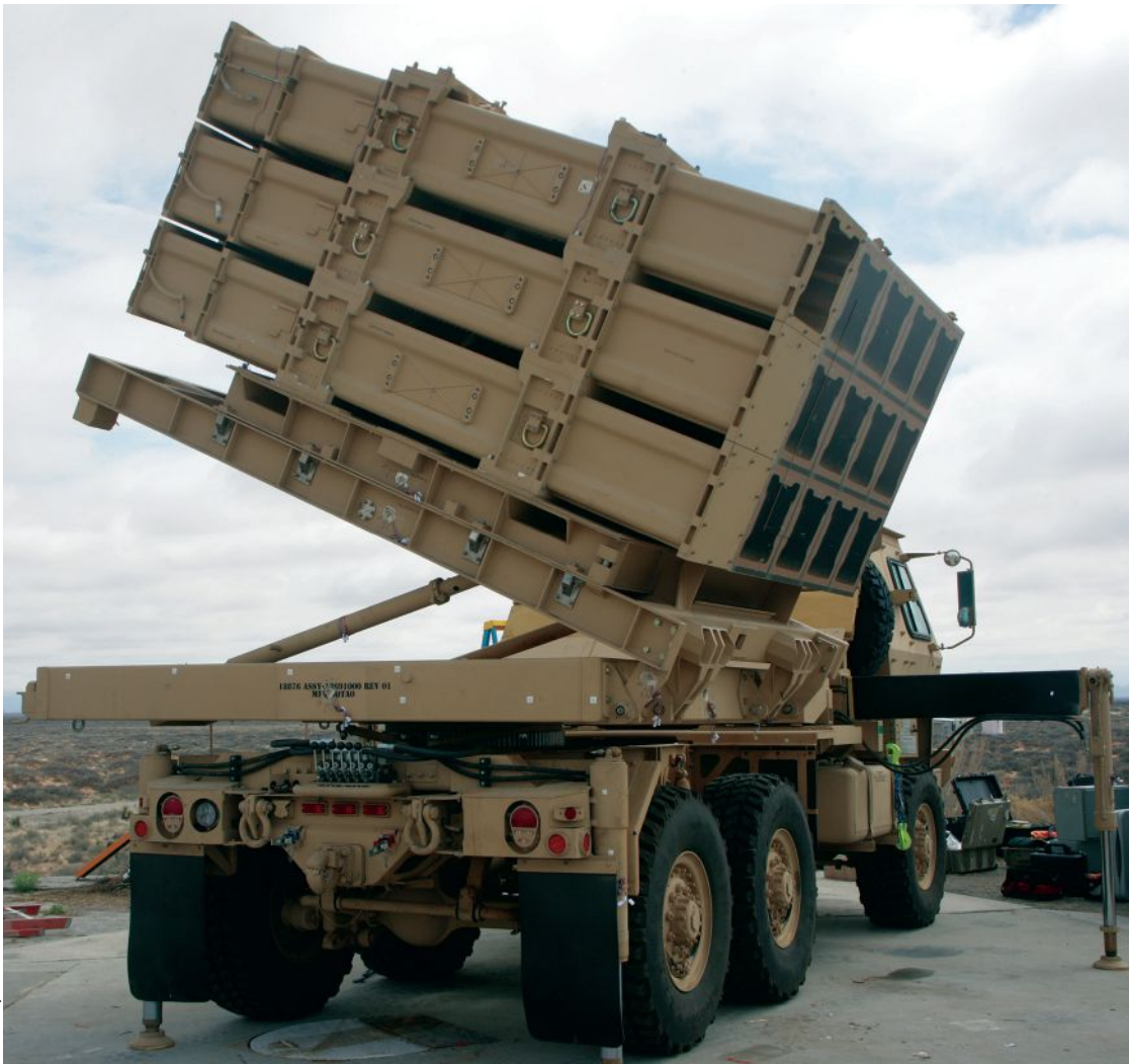
Mounted on a medium tactical truck, the multimission launcher can rotate 360 degrees and elevate to 90 degrees.
